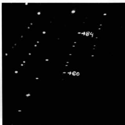
Fig. 6. Zero layer a -axis Weissenberg photograph of polytype 24H_g ; Cu K\alpha radiation; camera diameter 5.73 cm; the festoon corresponding to 10.l row of spots is recorded on the right side of the straight row of 00.l spots; the l -value of two strong spots is mentioned on the photograph.
