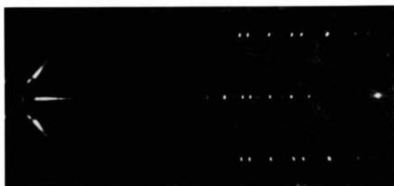
Fig. 4. A 15^\circ a -axis oscillation photograph of polytype 24H_g (crystal no. 2); 3 cm camera; Cu K\alpha radiation.
