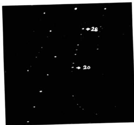
Fig. 3. Zero layer a -axis Weissenberg photograph of polytype 8H_b ; Cu K\alpha radiation; camera diameter 5.73 cm; the festoons corresponding to the 10.l and \bar{1}0.l rows of spots are recorded on the right and left side, respectively, of the straight row of 00.l spots; the l -value of two strong spots is mentioned on the photograph.
